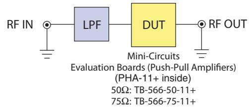
**Fig 1b.** Block Diagram of Test Set up used for characterization of Gain, IP2, IP3. Measured using Agilent’s signal generators E8527D and Spectrum analyzer N9020A.
