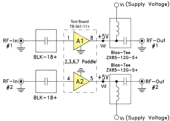
**Fig 1a.** Block Diagram of Test Circuit used for characterization. (DUT tested in Mini-Circuits Test board TB-561-11+, except for IP2) Gain, Return loss, Output power at 1dB compression (P1 dB), output IP3 (OIP3) and noise figure measured using Agilent’s N5242A PNA-X microwave network analyzer.
