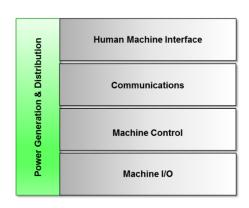
Alongside these four ingredients is the power generation and distribution system, often 12 or 24VDC supplied initially by 110/220VAC wall power.
