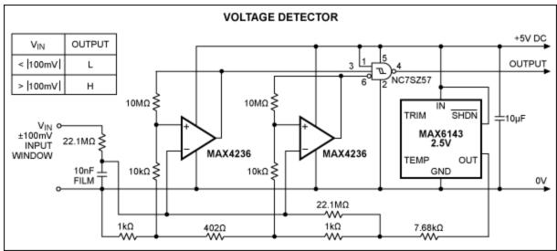
Figure 1. This detector of bipolar DC voltages asserts a digital output signal when the input is within a  $\pm 100$ mV window, centered at 0V.
