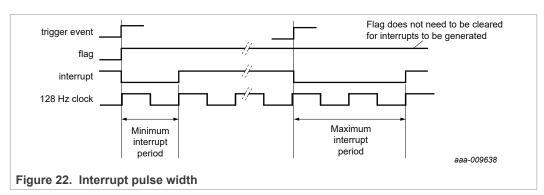
In level mode, the interrupt signal follows the state of the flag. Only interrupts which are enabled will affect the pin state. All enabled flags must be cleared for the interrupt signal to be cleared.
