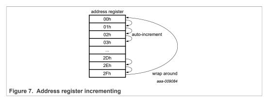
All registers (see <u>Table 4</u>, <u>Table 5</u>, and <u>Table 6</u>) are designed as addressable 8-bit parallel registers although not all bits are implemented. <u>Figure 8</u> gives an overview of the address map.
