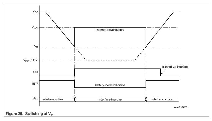
7.11.3.2 Switching at the  $V_{BAT}$  level, BSM[1:0] = 01
