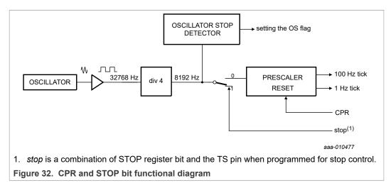
The *stop* signal blocks the 8.192 kHz clock from generating system clocks and freezes the time. In this state, the prescaler can be cleared with the CPR command in the Resets register (Section 7.15).
