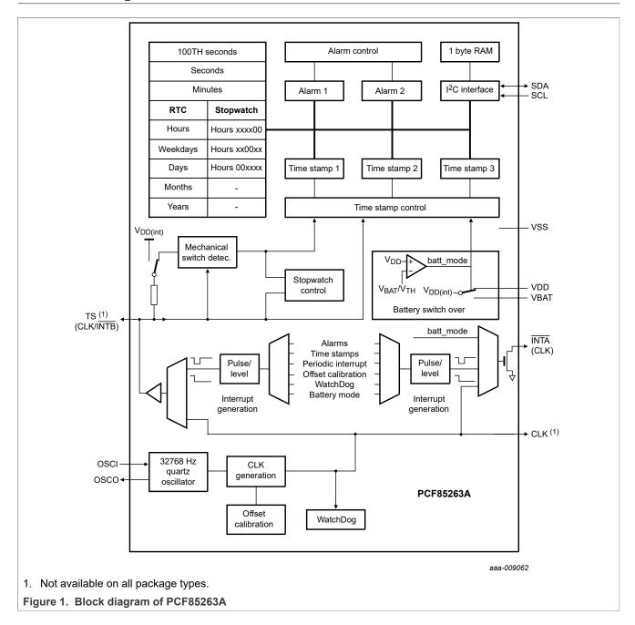
Tiny Real-Time Clock/calendar with alarm function, battery switch-over, time stamp input, and I<sup>2</sup>C-bus
