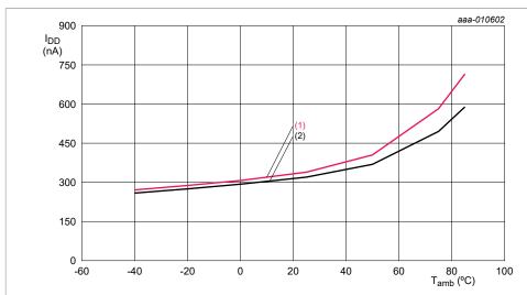
$C_{L(itg)}$  = 7 pF; CLKOUT disabled; battery switched on.
