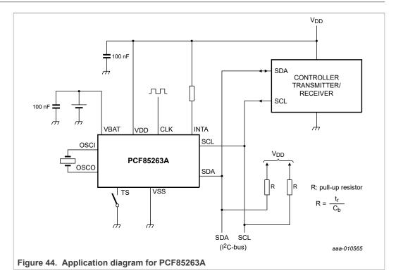
The data sheet values were obtained using a crystal with an ESR of 60 k $\Omega$ . If a crystal with an ESR of 70 k $\Omega$  is used then the power consumption would increase by a few nA and the start-up time will increase slightly.
