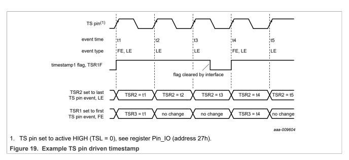
The recorded time is stored in the associated timestamp register. The time format depends on the RTC mode. The timestamp registers follows the time format of the time registers.
