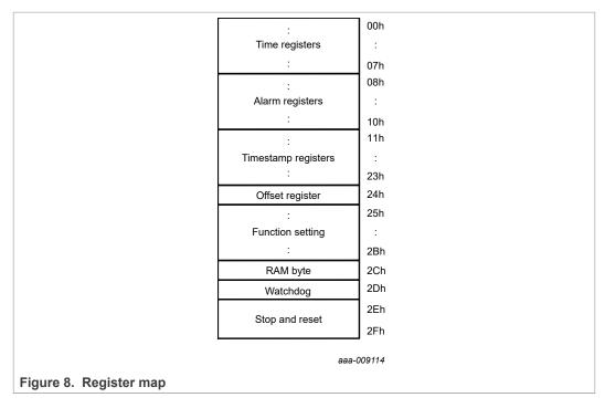
The 100th seconds, seconds, minutes, hours, days, months, and years as well as the corresponding alarm registers are all coded in Binary Coded Decimal (BCD) format. When one of the RTC registers is read, the contents of all time counters are frozen. Therefore, faulty reading of the clock and calendar during a carry condition is prevented.
