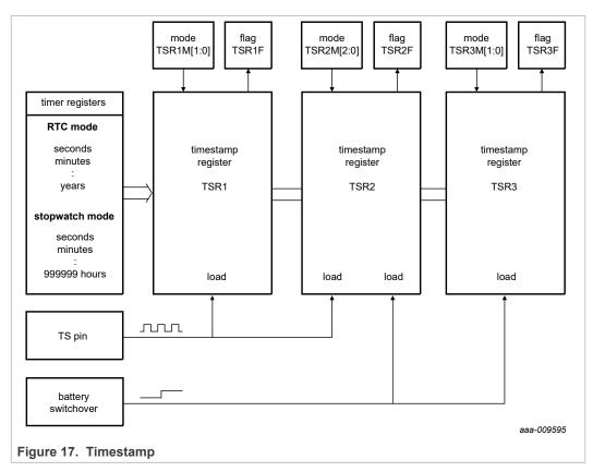
The mode for each register is controlled by the TSR\_mode register.
