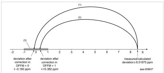
With the offset calibration an accuracy of  $\pm 1$  ppm (0.5 × offset per LSB) can be reached (see Table 24).
