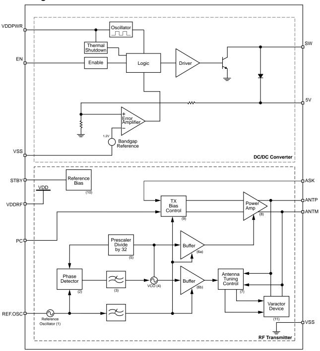
Figure 2. MICRF104 Block Diagram (RF Circuit)
