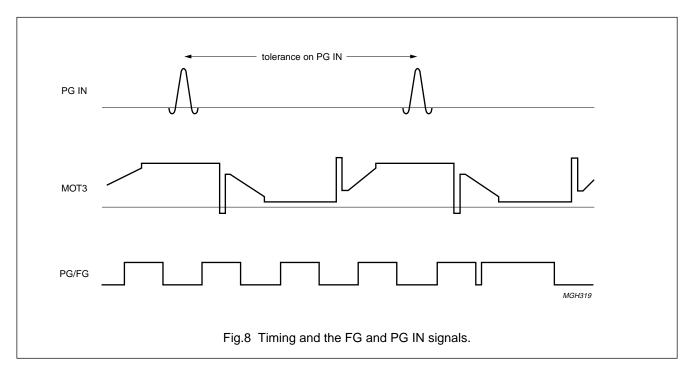
The special PG pulse is derived from the negative-going zero-crossing from the MOT3 output (pin 16). The external PG signal (PG IN on pin 5) must sense a positive-going voltage (>80 mV) within 1.5 to 7.5 commutation periods before the negative-going zero-crossing in MOT3 (see Fig.8).
