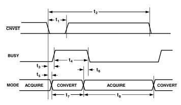
Figure 8. Basic Conversion Timing
