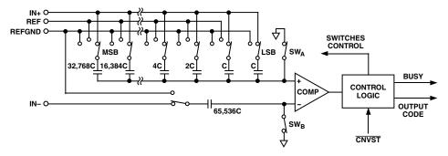
Figure 3. ADC Simplified Schematic
