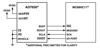
Figure 18. Interfacing the AD7650 to SPI Interface
