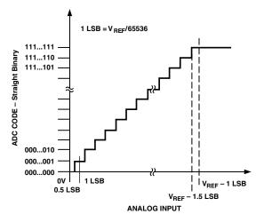
Figure 4. ADC Ideal Transfer Function
