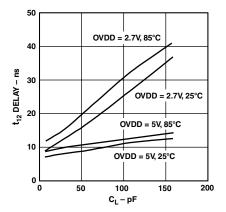
TPC 9. Typical Delay vs. Load Capacitance  $C_L$
