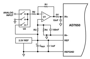
Figure 20. Using the AD7650 in 16-Bit Bipolar and/or Wider Input Ranges
