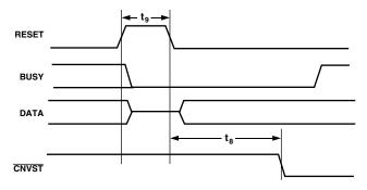
Figure 9. RESET Timing
