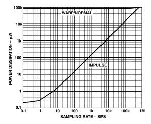
Figure 7. Power Dissipation vs. Sampling Rate
