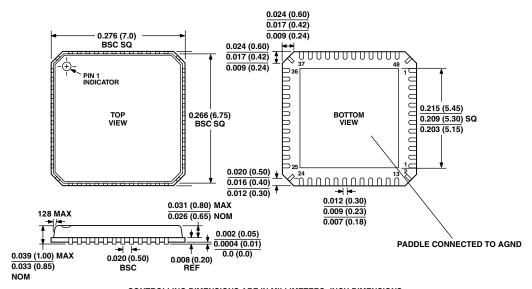
CONTROLLING DIMENSIONS ARE IN MILLIMETERS; INCH DIMENSIONS ARE ROUNDED-OFF MILLIMETER EQUIVALENTS FOR REFERENCE ONLY AND ARE NOT APPROPRIATE FOR USE IN DESIGN
