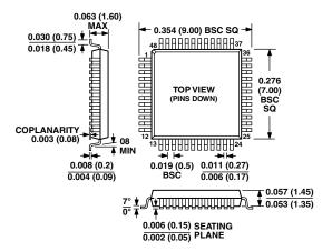
CONTROLLING DIMENSIONS ARE IN MILLIMETERS; INCH DIMENSIONS ARE ROUNDED-OFF MILLIMETER EQUIVALENTS FOR REFERENCE ONLY AND ARE NOT APPROPRIATE FOR USE IN DESIGN
