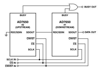
Figure 17. Two AD7650s in a "Daisy-Chain" Configuration
