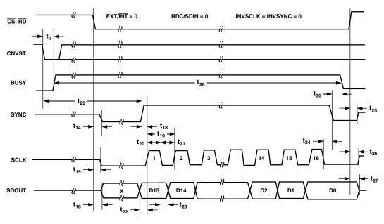
Figure 13. Master Serial Data Timing for Reading (Read After Convert)
