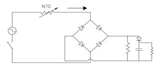
Ct2 Test capacitance [µF] Imax2 Max current across the NTC under test [A] Number of cycles: 1000
