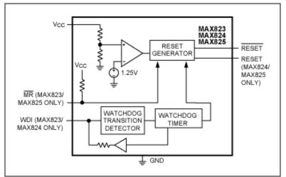
Figure 6. The MAX823-MAX825 family integrates two popular functions: watchdog and reset. Factory-Preset Watchdog Families
