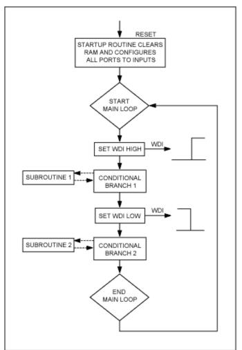
Figure 5. An improved program flow has two separate watchdog-toggle commands, which generate a rising-and a falling-edge signal on the WDI pin. This prevents the program from being stuck in a parasitic loop.
