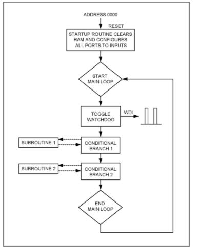
Figure 2. This figure shows a typical program flow with the WDI signal generated within the main loop.
