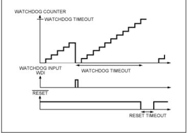
Figure 4. As soon as the watchdog counter reaches the timeout value, a reset is generated.
