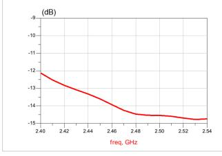
Figure 4. Return loss on DIFF port (T<sub>amb</sub> = 25 °C)
