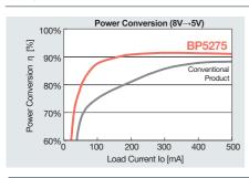
Conversion efficiency is significantly increased over conventional products, making it easy to lower set power consumption. In addition, the output voltage is accurate to within ±2%.
