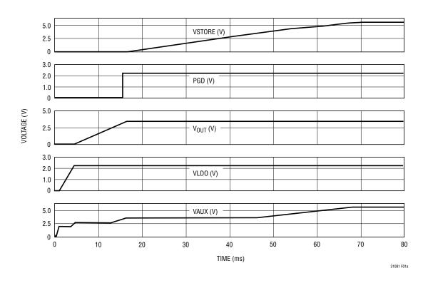
Figure 1. Output Voltage Sequencing with  $V_{OUT}$  Programmed for 3V (Time Not to Scale)
