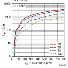
I<sub>VOUT</sub> vs V<sub>IN</sub> and Source Resistance, 1:100 Ratio
