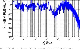
Figure 3: Typical output noise voltage spectral density  $e_{no}$ with  $R_{\rm M}$  = 100  $\Omega$
