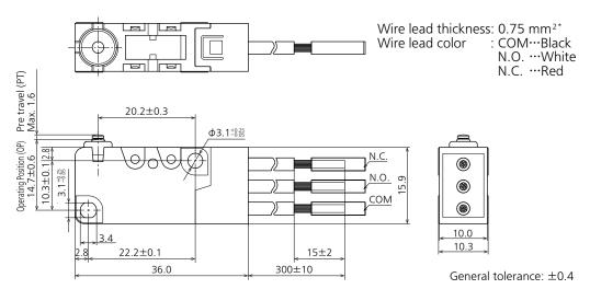
Note) Dimensions of the actuator types are the same as those of corresponding solder and .187 quick–connect terminal types. \* With UL and CSA approved products, lead wire is changed to UL compliant (AWG18).
