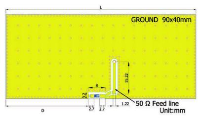
The minimum sie for VJ5106W240 is L > 30 mm and D > 6 mm
