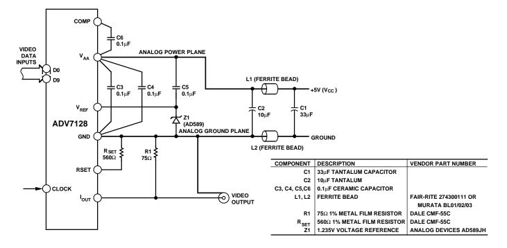
Figure 7. ADV7128 Typical Connection Diagram and Component List
