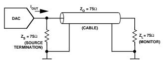
Figure 5a. Analog Output Termination for RS-343A
