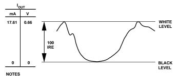
1. OUTPUTS CONNECTED TO A DOUBLY TERMINATED 75 $\Omega$  LOAD.
