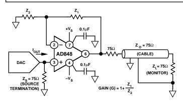
Figure 6. AD848 As an Output Buffer
