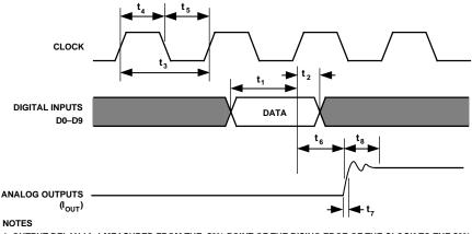
1. OUTPUT DELAY (  $\rm f_6$  ) MEASURED FROM THE 50% POINT OF THE RISING EDGE OF THE CLOCK TO THE 50% POINT OF FULL-SCALE TRANSITION.
