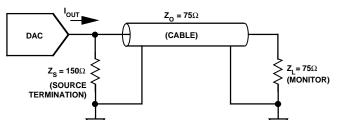
Figure 5b. Analog Output Termination for RS-170
