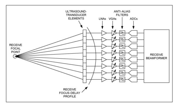
Figure 7. Signals from each transducer element are amplified and digitized by receive channels in the ultrasound-receiver system.
