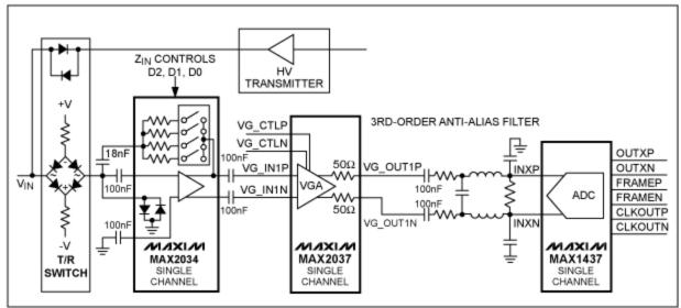
Figure 1. A typical phased-array ultrasound-receiver lineup consists of an LGA, a VGA, an anti-alias filter, and an ADC.
