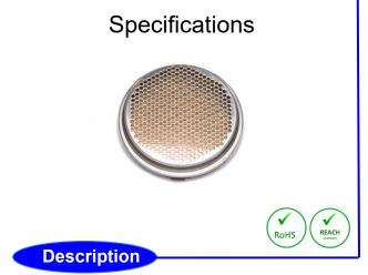
The Series 600 ultra-sensitive ultrasonic sensors feature ranging capability from 2.5 cm to 15.2 m when used with SensComp drive electronics. They are ideally suited for demanding applications where the most sensitivity possible is the highest priority. These ultrasonic sensors are among the best available when detecting soft targets. They have a broad band frequency response.
