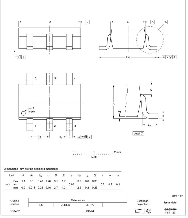
Fig. 8. Package outline SOT457 (SC-74; TSOP6)
