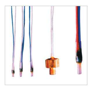
**PTC Thermistors** act as thermal protectors for electrical motors. They are available with or without an insulated sleeve and have flexible connecting leads. PTC thermistors have a non-linear resistance/temperature response. At a specified temperature the resistance changes rapidly to a very high value.
