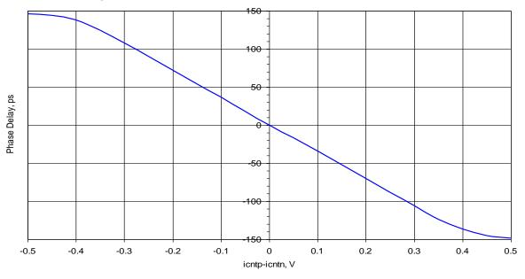
Fig. 2. Delay Control Diagram
