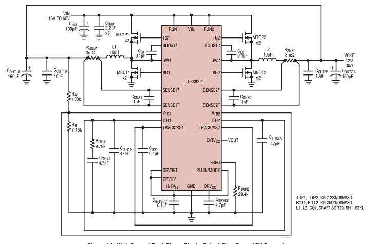
Figure 14. High Current Dual-Phase Single Output Step-Down 12V Converter
