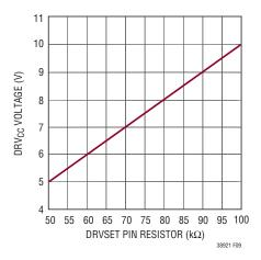
Figure 8. Relationship Between DRV<sub>CC</sub> Voltage and Resistor Value at DRVSET Pin
