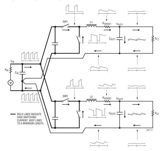
Figure 10. Branch Current Waveforms
