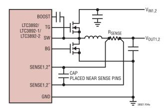
(2a) Using a Resistor to Sense Current
