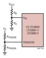
Figure 7. Using the TRACK/SS Pin for Tracking
