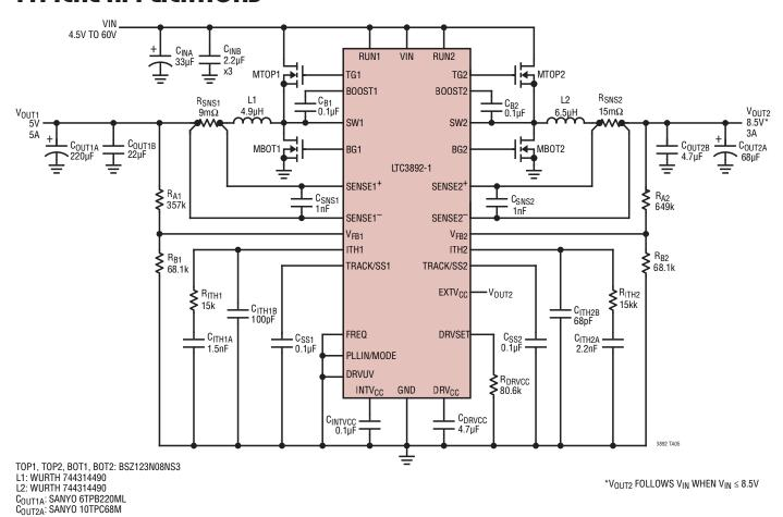
Figure 13. High Efficiency Dual-Phase Step-Down 5V/8.5V Converter with 8V Gate Drive
