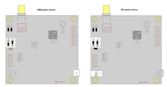
Figure 4: USB and DC 3.6 V to 5.5 V power source jumper connections
