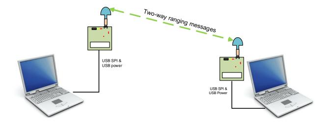
Figure 17: Both EVB1000's controlled by the external application
