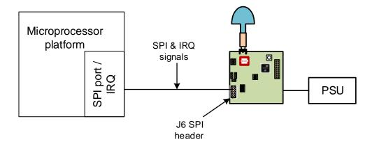
Figure 16: External application control with a microprocessor platform using SPI external header
