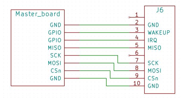
Figure 20 EVB1000 External control connectivity
