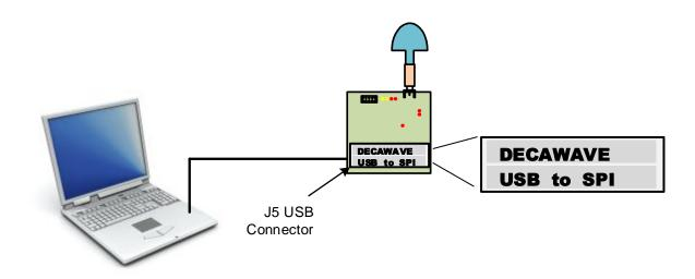
Figure 13: External application control using USB interface
