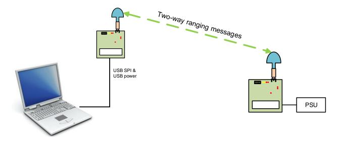
Figure 18: One EVB1000 controlled by the external application
