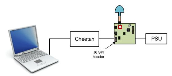
Figure 15: External application control using SPI external header
