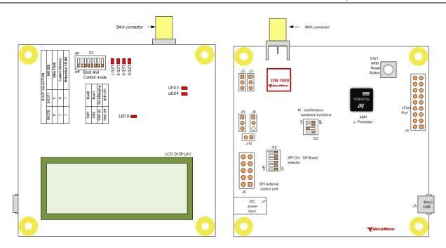
Figure 2: The two sides of the EVB1000 showing main components
