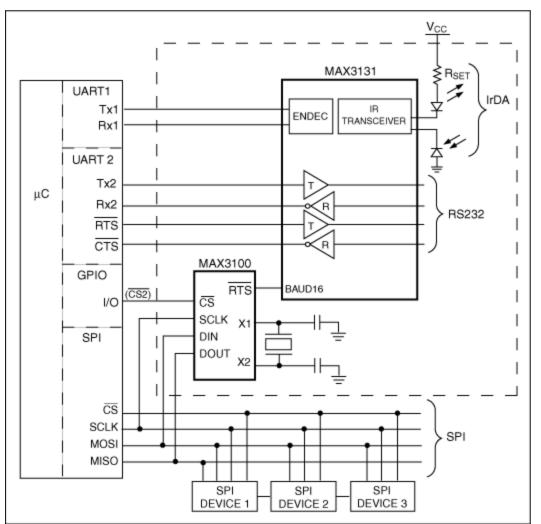
Figure 7. This MAX3100 circuit requires only one additional  $\mu$ C I/O to implement a software-adjustable BAUD16 clock generator.
